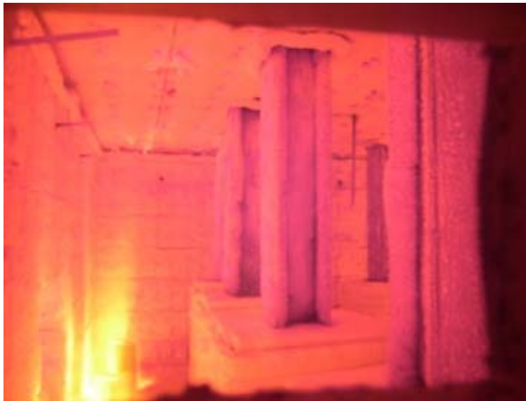
Char forming (W8x31 in center of picture)
