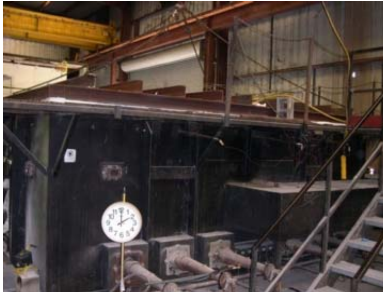
Furnace extinguished after 2 hours of exposure
