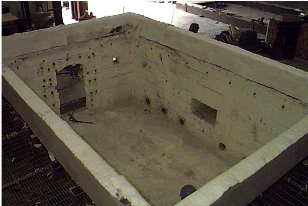
12' x 18' Horizontal Fire Resistance Furnace
