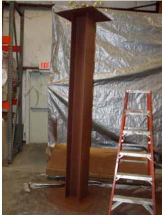
#1: Primed column ready to coat.
