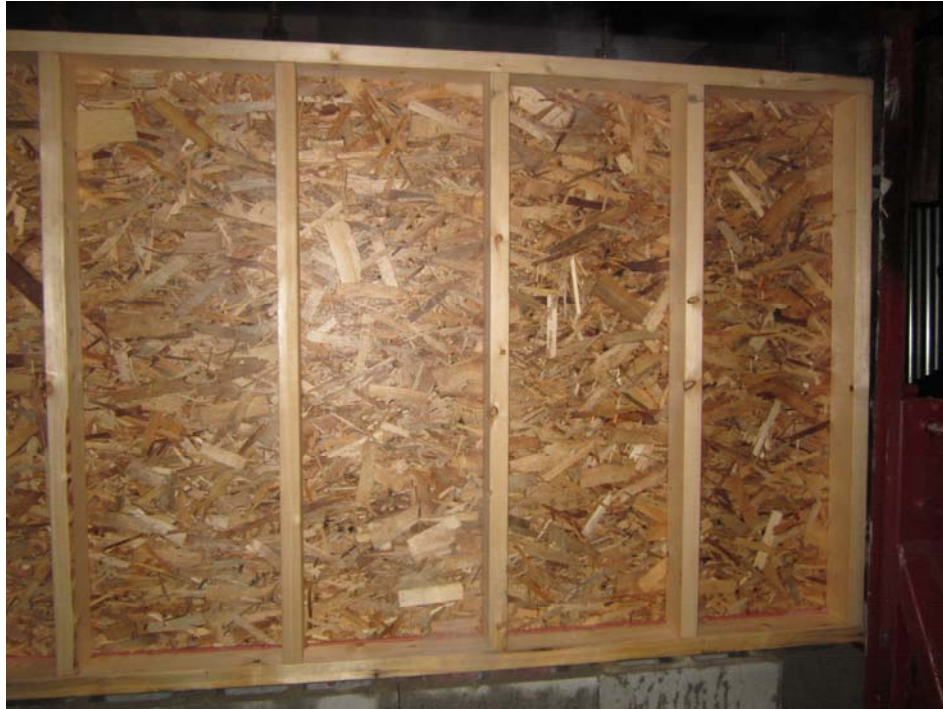
Unexposed Side During the Fire Test at 15 Minutes
