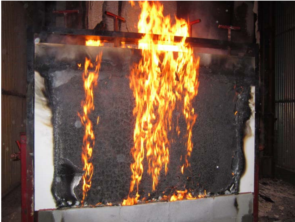
Exposed Side After the Fire Test
