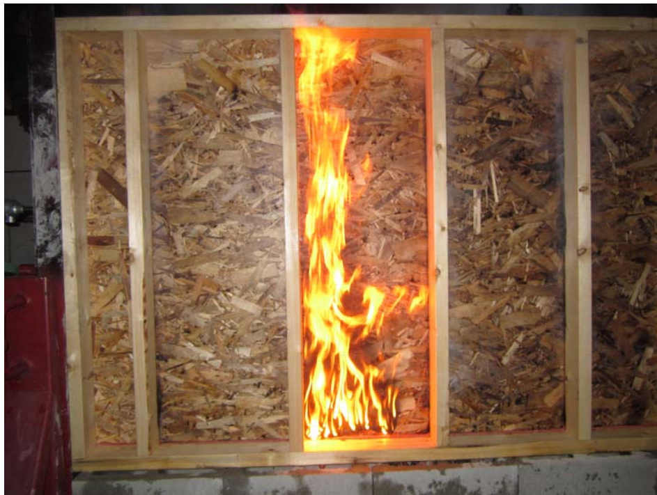
Unexposed Side After the Failure of the Fire Test
