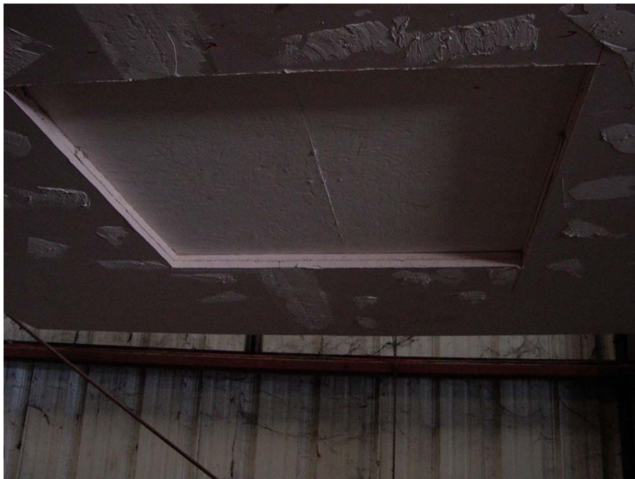
Sample mounted in the test frame prior to mounting on the furnace
